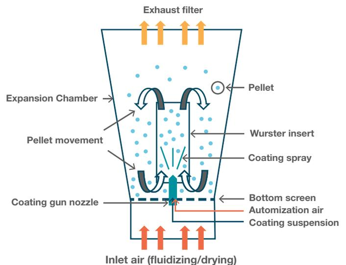
The liquid spray may be an aqueous- or solvent-based solution, a suspension, or a melt. In a well-controlled process, each particle receives a similar quantity of coating, resulting in a uniform population of coated particles. Multi-step processes in which the same or different coatings are layered to achieve desired film thickness and functionality increase the range of possibilities.
